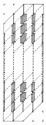
FIGURE 8. Structure of the 13-diagonal banded coefficient matrix.
