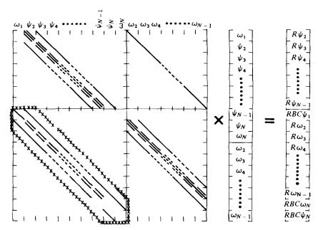
FIGURE 7. Structure of the linear system in Newton's method.
