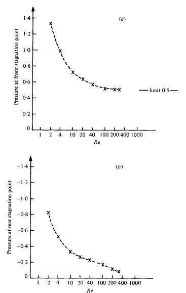
FIGURE 19. The pressure at (a) the front stagnation point and (b) the rear stagnation point.
