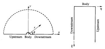
FIGURE 1. The x, y and  $\xi$ ,  $\eta$  plane.
