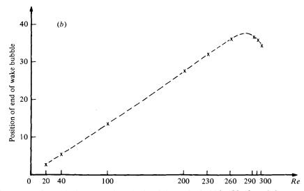
FIGURE 17. The width (a) and length (b) of the wake bubble. The length is measured from the centre of the cylinder.
