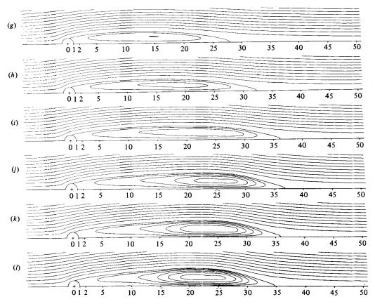
FIGURE 10. Streamlines at different Reynolds numbers. (a) Re = 2; (b) Re = 4; (c) Re = 10; (d) Re = 20; (e) Re = 40; (f) Re = 100; (g) Re = 200; (h) Re = 230; (i) Re = 260; (j) Re = 290; (k) Re = 295; (l) Re = 300.
