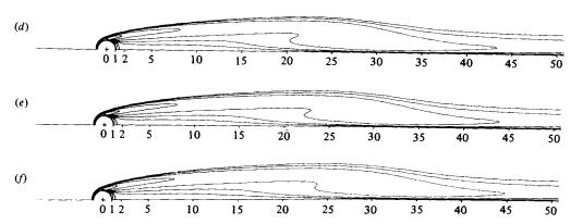
FIGURE 13. Numerical solution at Re = 290 for different values of the parameter c in the mapping for the inner grid. (a) c = 0.2, (b) c = 0.25, (c) c = 0.3, (d) c = 0.2, (e) c = 0.25, (f) c = 0.3.
