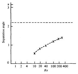
FIGURE 16. The position of the separation point.
