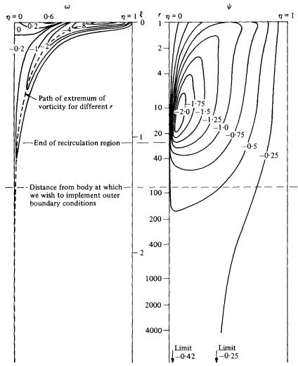
FIGURE 5. Contours of  $\omega$  and  $\psi$  at Re=200.
