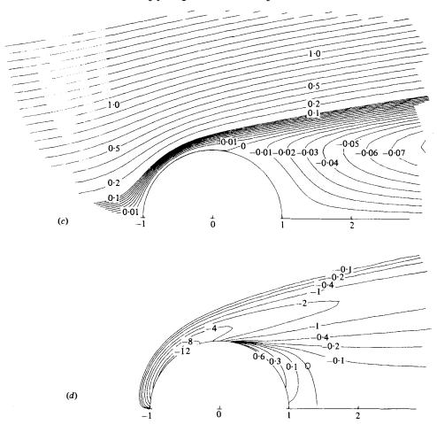
Figure 14. Details of the flow pictures for Re = 20 and Re = 20. Re = 20, (a) stream function, (b) vorticity. Re = 200, (c) stream function, (d) vorticity.
