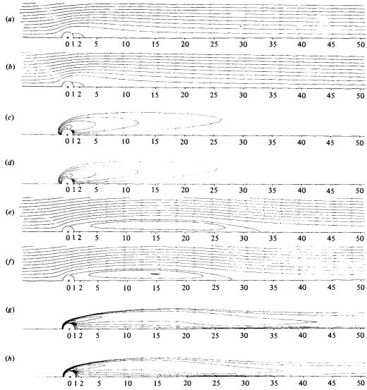
FIGURE 12. Comparison between results on coarse and fine computational grids. Re = 20, (a) coarse grid, (b) fine grid, (c) coarse grid, (d) fine grid. Re = 200, (e) coarse grid, (f) fine grid, (g) coarse grid, (h) fine grid.
